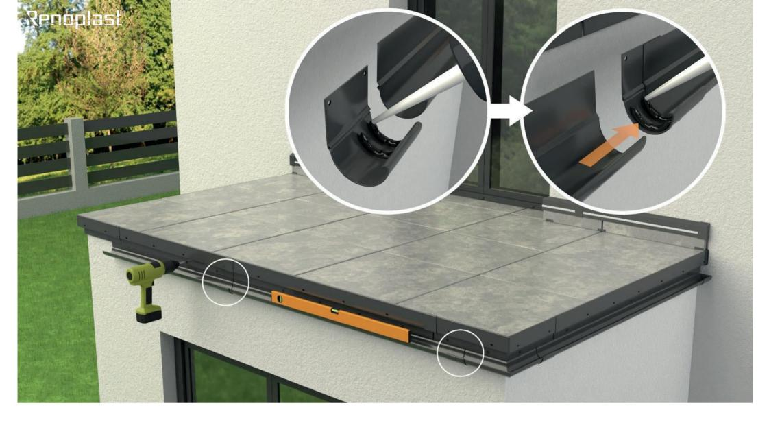
Installation of subsequent sections of the R50 gutter to the eaves profile
