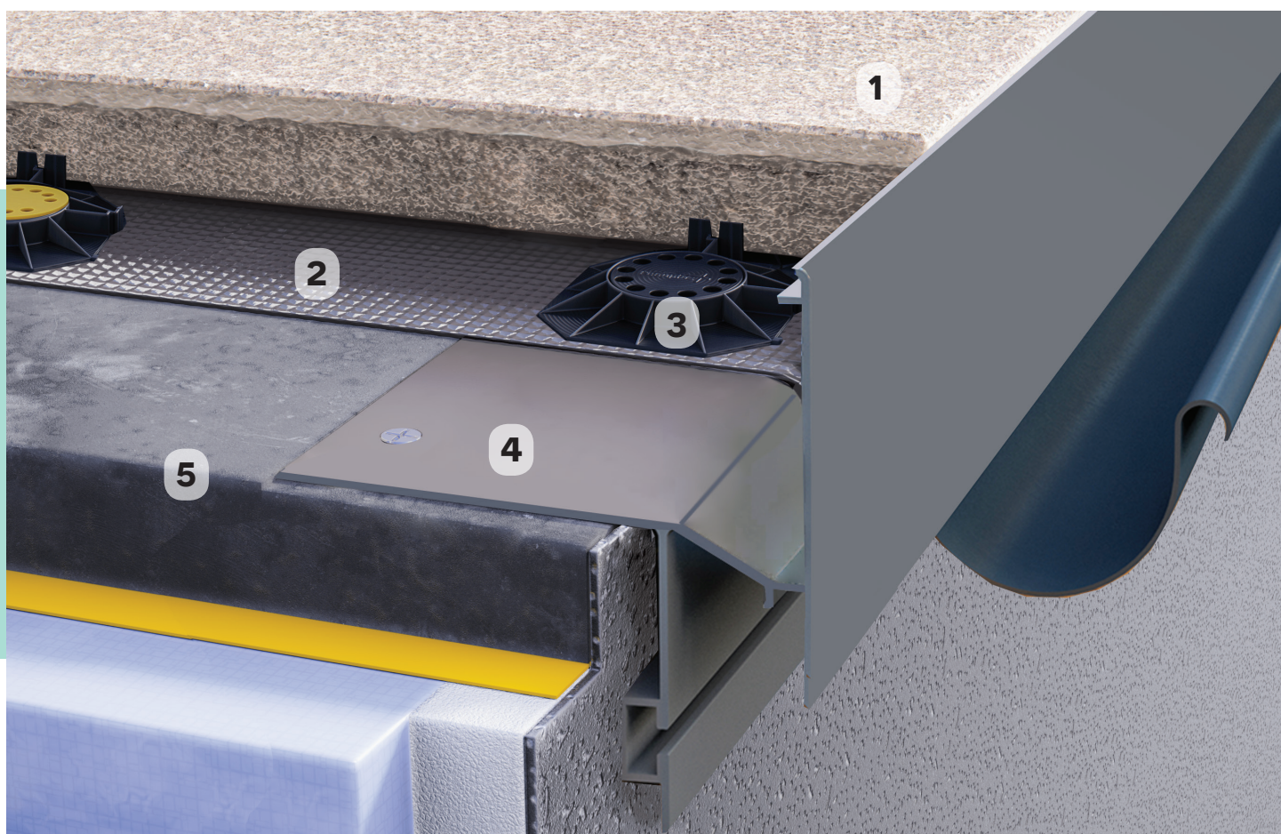
1. STONEWARE, STONE OR CONCRETE SLABS; 2. WATERPROOFING; 3. SMART PAD; 4. K60 HOOD PROFILE; 5. CEMENT PRIMER;
